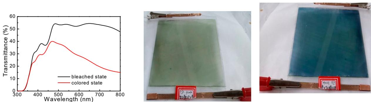
**Figure 7.** Transmittance spectra and corresponding digital photos of PANI/ $\text{WO}_3$  assembled device in bleached and colored states.
