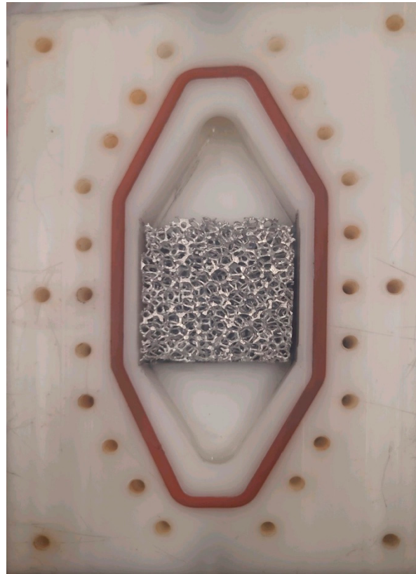
Figure 3. Metal foam porous material in the test section.
