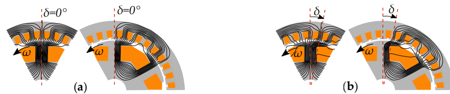
Figure 4. Load angle of a synchronous machine, in this case a generator with the rotor flux leading the stator flux. Showing: (a) A no-load case \delta = 0^\circ . (b) A case with a load \delta \neq 0^\circ .
