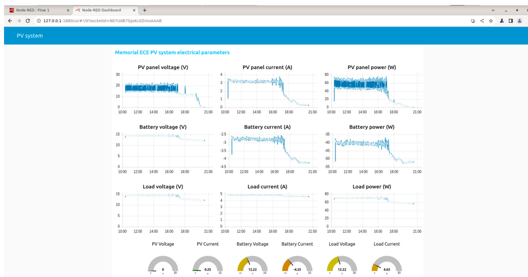
Figure 12. Node-RED dashboards showing the monitored values of the PV system.
