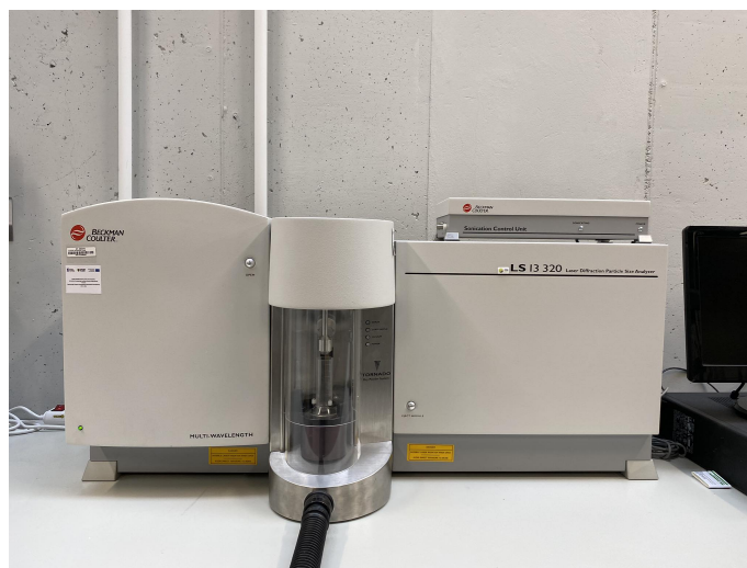
Figure 5. LS 13 320 particle size analyzer for milling product granulometry.
