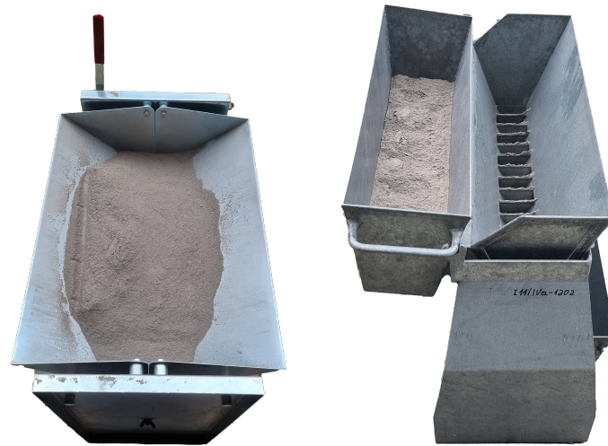
Figure 4. Jones splitter for sample preparation.
