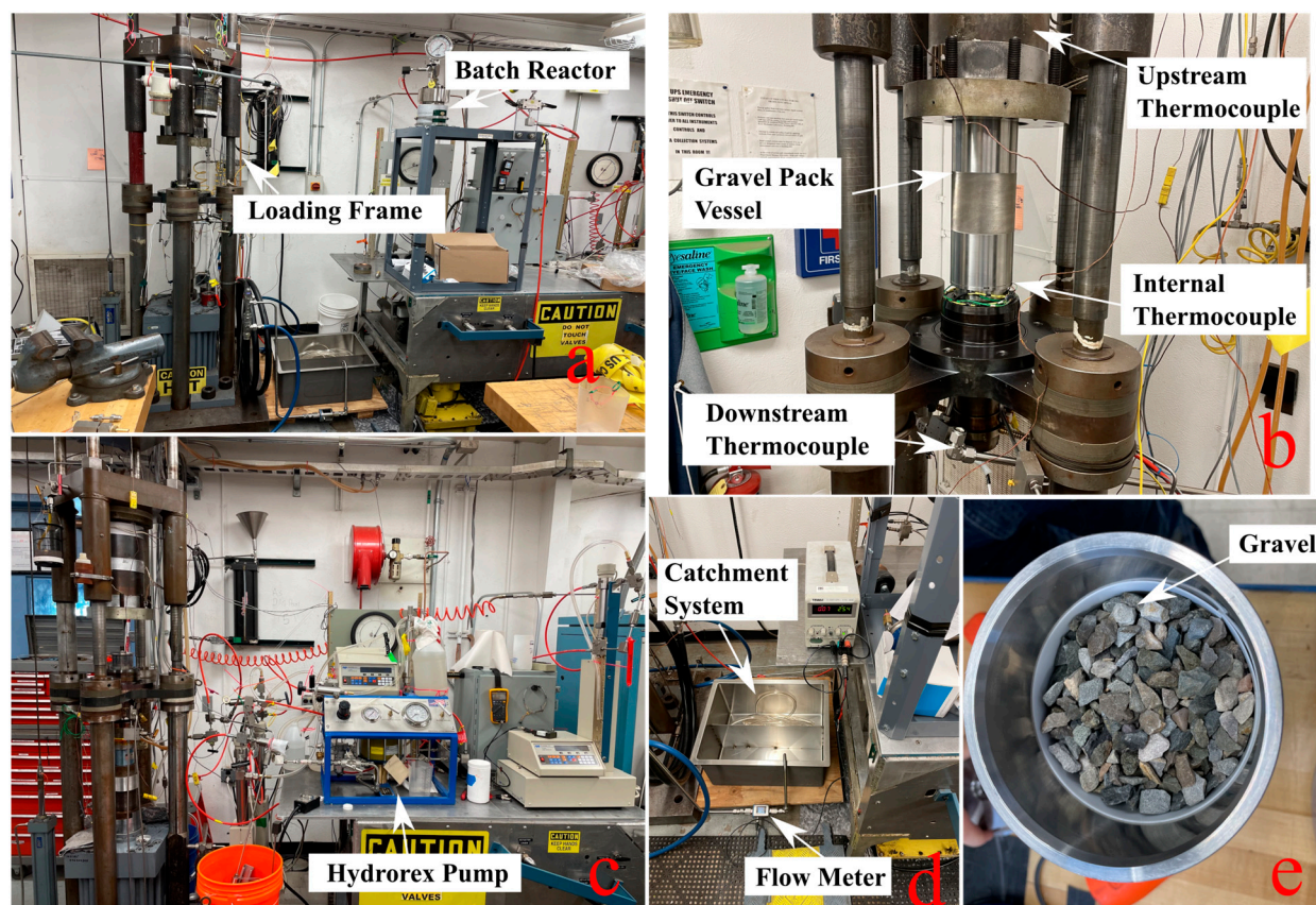
Figure 6. Photos of flow loop system equipment showing: (a) the empty testing frame and batch reactor; (b) gravel pack cylinder in testing frame; (c) Hydrex pressure system for maintaining constant flow through; (d) flow meter and catchment tank for removing LCMs that pass through gravel pack; (e) untested gravel pack showing gravel and Teflon covering inside.
