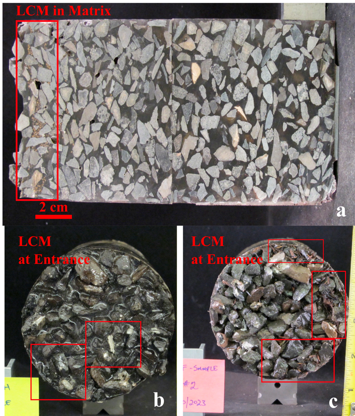
Figure 15. LCM trapped in epoxied samples: (a) FMC + CMC trapped in matrix; (b) SD + CSH trapped at the entrance to the matrix; (c) CMC + CF trapped in the matrix entrance. Direction of flow through gravel pack in (a) is from left to right; entrance to gravel pack is shown in both (b,c). Red boxes indicate where trapped LCM can be seen in the epoxied samples.
