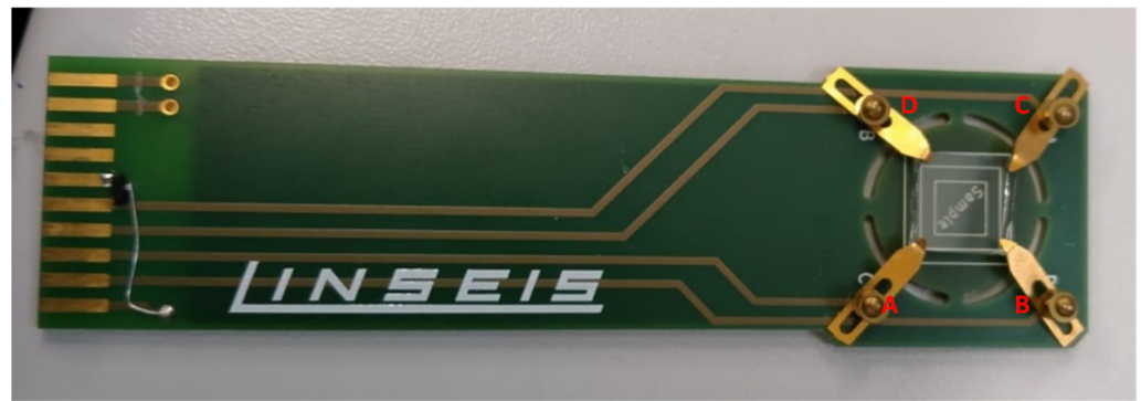
Figure 1. A sample with dimensions of 10 \times 10 \text{ mm}^2 was mounted in the sample holder.
