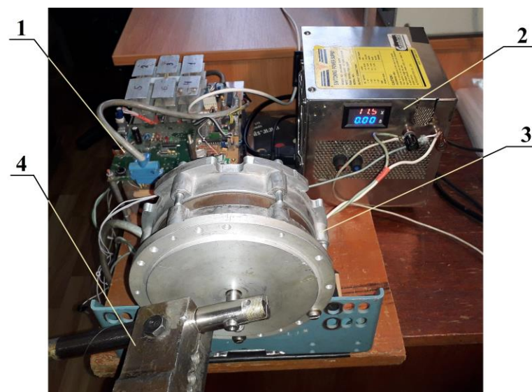
Figure 8. Laboratory setup designed to research PMSM motor under variable load: (1) PLL inverter; (2) DC source; (3) PMSM motor; (4) variable load imitator.
