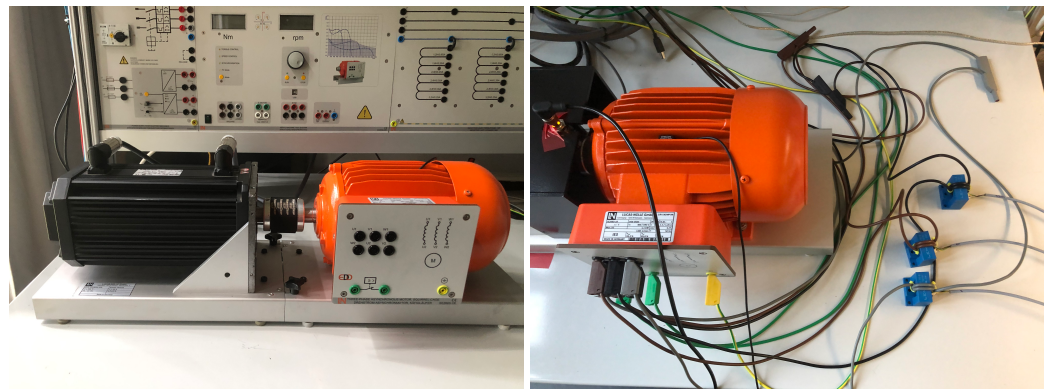
Figure 6. Example machine in the form of a 1.1 kW squirrel cage induction motor (shaft protection removed for better visibility of the coupling) with test bench in the background ( left ) and example machine together with current transformers ( right ).
