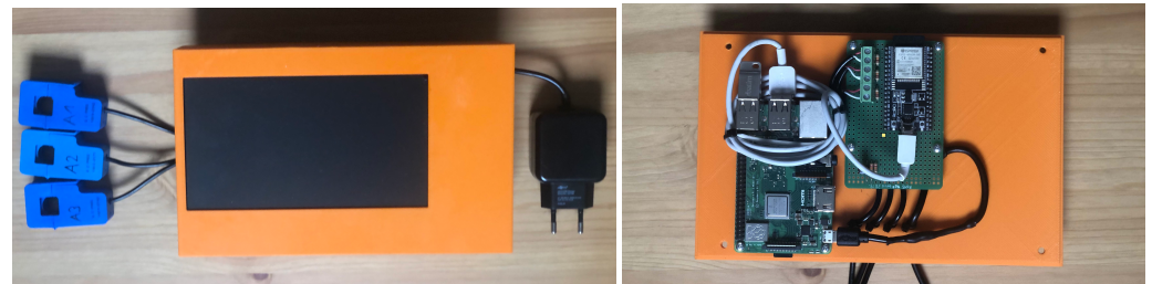
Figure 13. Monitoring system with orange housing, LED display, current transformers and power supply (left), and open housing with Raspberry Pi and ESP32 microcontroller (right).
