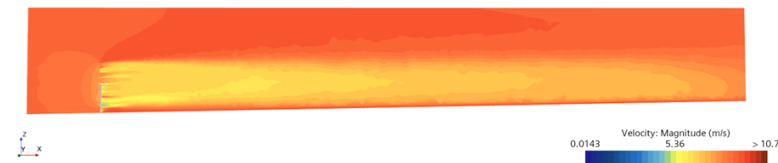
Figure 10. Speed distribution scene in the computational domain behind the simulated wind turbine.
