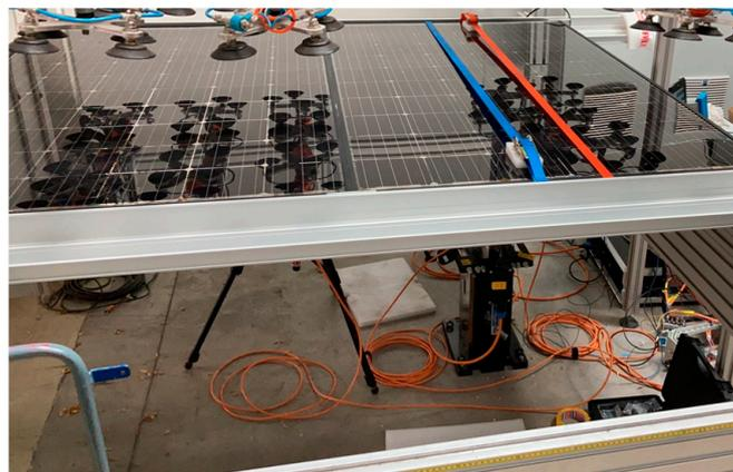
**Figure 18.** Vibration-test setup, top view.
