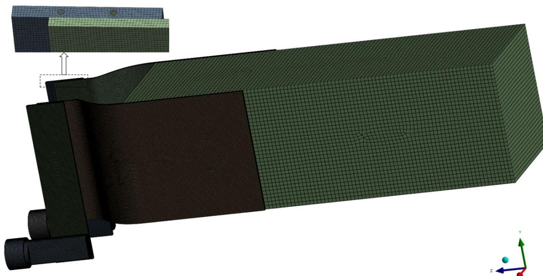
Figure 4. Mesh of the numerical model.
