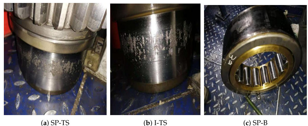
Figure 8. Examples of the faults found in WT No. 25. ((a) Spalling on the high-speed shaft tooth surface (SP-TS), (b) Indentation of the high-speed shaft tooth surface (I-TS), and (c) Spalling on the high-speed shaft bearing (SP-B)).
