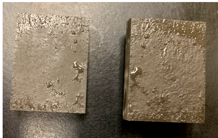
Figure 3. Image of fracture surfaces of core plug Sample #3. This core plug was fractured during the oil saturation stage.
