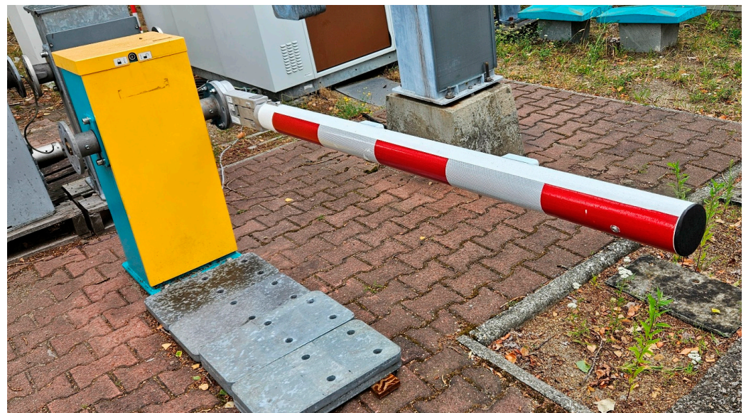
Figure 24. EEG-3 drive with proprietary BLDC motor during field testing.
