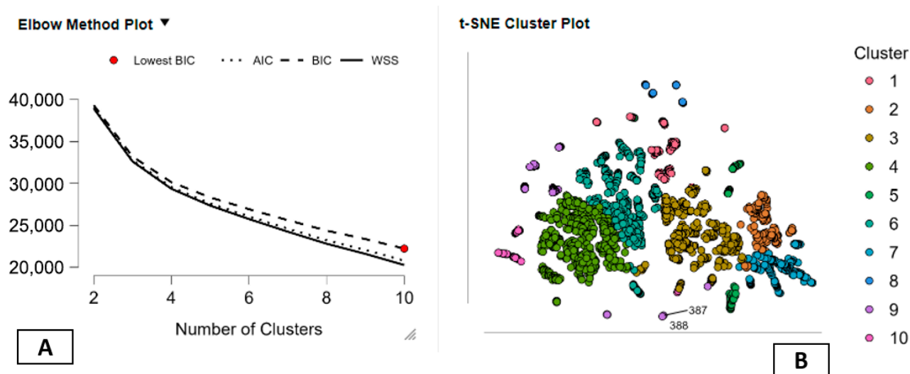
Figure 2. Determination and validation of optimal clusters in K-Means analysis of cross-country energy use. Note: Panel (A) shows the Elbow Method using WSS, AIC, and BIC to identify the optimal number of clusters, with the minimum BIC indicating ten clusters as the best balance between goodness of fit and model complexity. Panel (B) presents a t-SNE visualization of the
