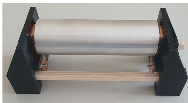
Figure 4. Surrogate model. Aluminum EN AW-2017 cylinder. R = 7 \mu\Omega .
