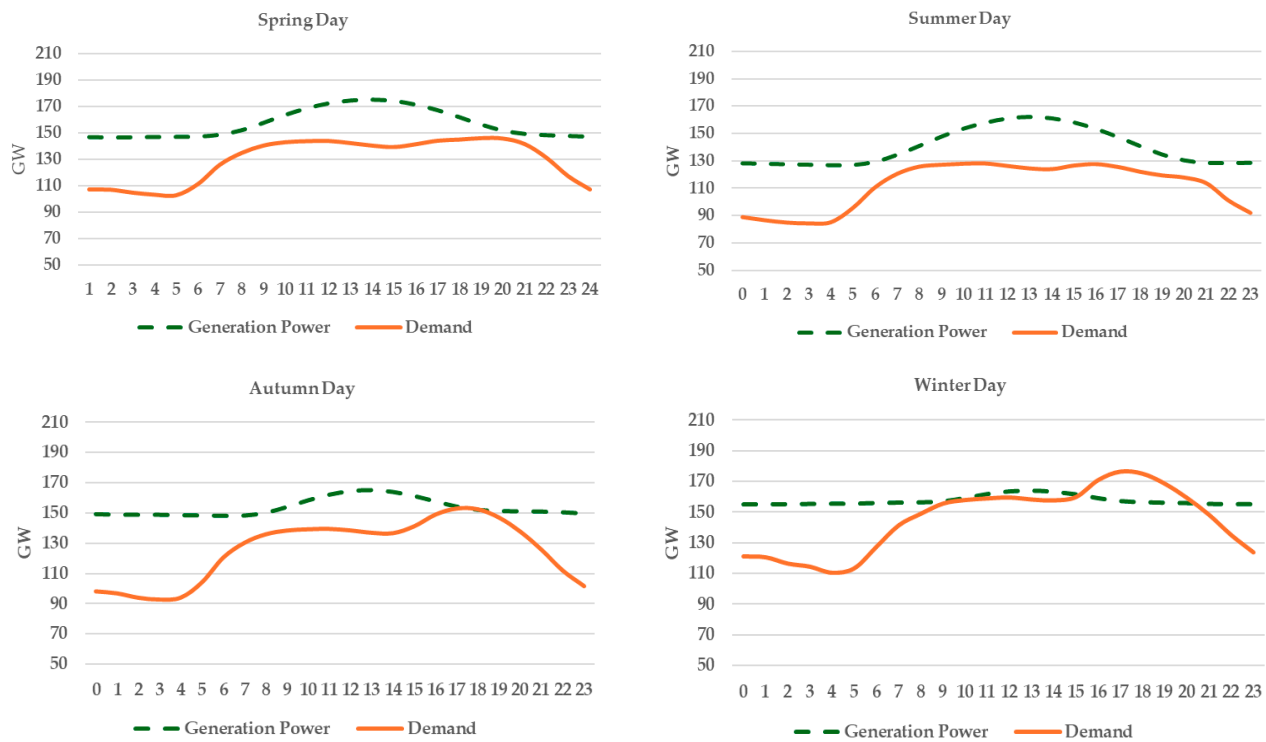
Figure A1. Co-development scenario: Average hourly demand and generation in each season. On average, electricity generation exceeds demand except for a short window of up to 5 h on winter evenings.
