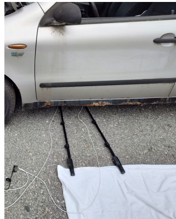
Figure 5. Arrangement of infrared sensors for upstream and downstream catalytic-converter-housing temperature monitoring.
