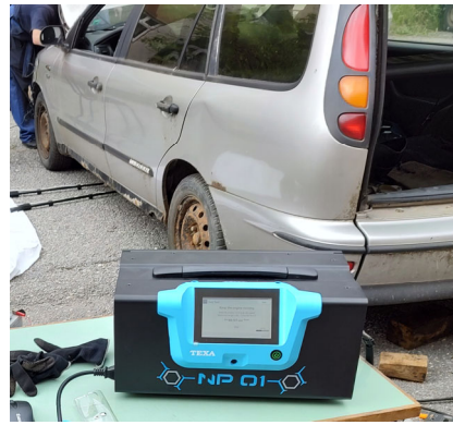
Figure 3. Diffusion charging (DC) particle number concentration (PNC).
