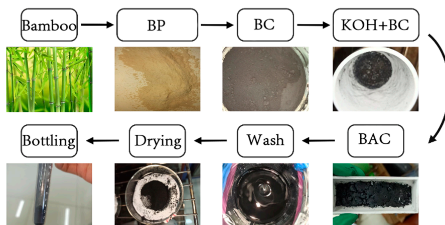
Figure 1. Schematic diagram of preparation of BAC.
