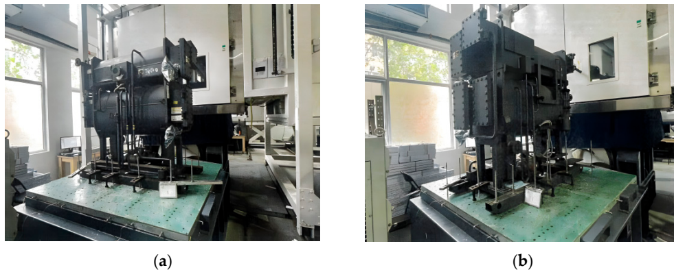
Figure 4. Vibration testing of LiBr absorption refrigeration units. (a) X-axis vibration; (b) Y-axis vibration.
