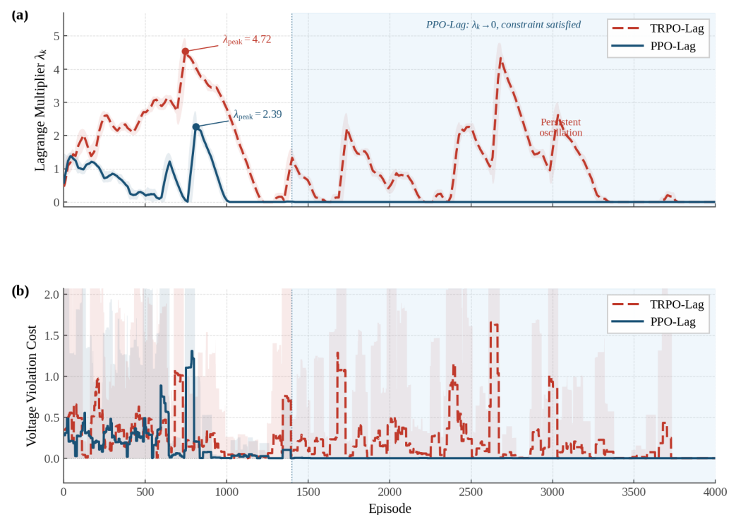
Figure 7. Comparison of training process between PPO-Lag and TRPO-Lag: (a) Lagrange multiplier \lambda_k trajectory; (b) Voltage violation cost trajectory.
