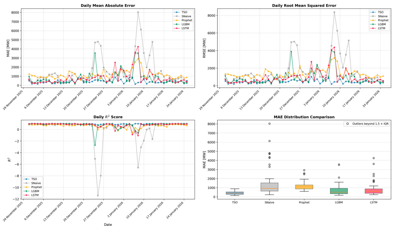
Figure 2. Daily error metrics (MAE, RMSE) and daily R^2 for 15 min load forecasts, with a boxplot of the daily MAE distribution, comparing TSO, SNaive, Prophet, LSTM, and LightGBM.
