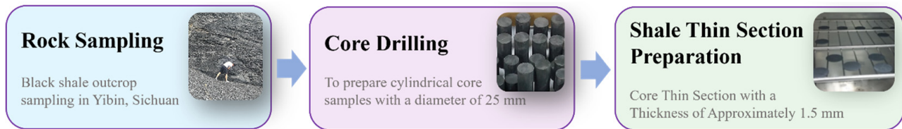
Figure 1. Sampling and Preparation of Rock Samples.
