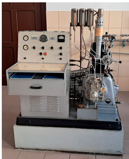
Figure 1. Test bench for measuring the cetane number of diesel.
