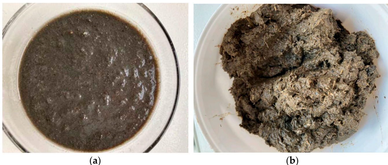
Figure 2. A mixture of primary and excess sludge in a 3:1 ratio (SS) (a) and cattle slaughterhouse waste (CSW) (b) (authors' own photographs).
