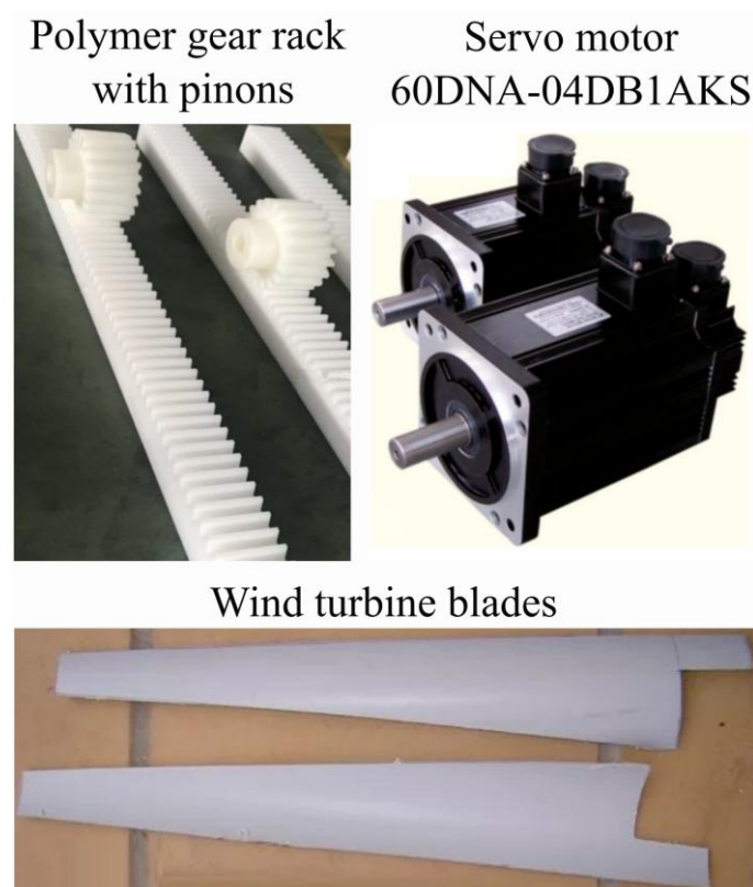
Figure 3. Photographs showing the polymer gear rack with its pinons, servo motor 60DNA-04DB1AKS, and the fabricated wind turbine blades.
