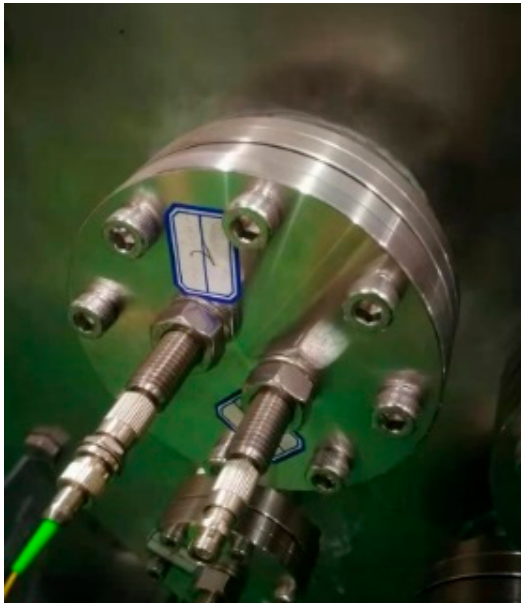
Figure 4. Installation method of fiber feedthrough.
