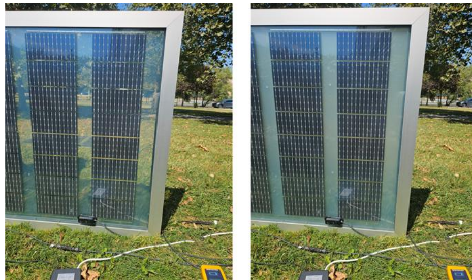
Figure 4. Transparent and opaque states in the testing phases of smart glass PV modules.
