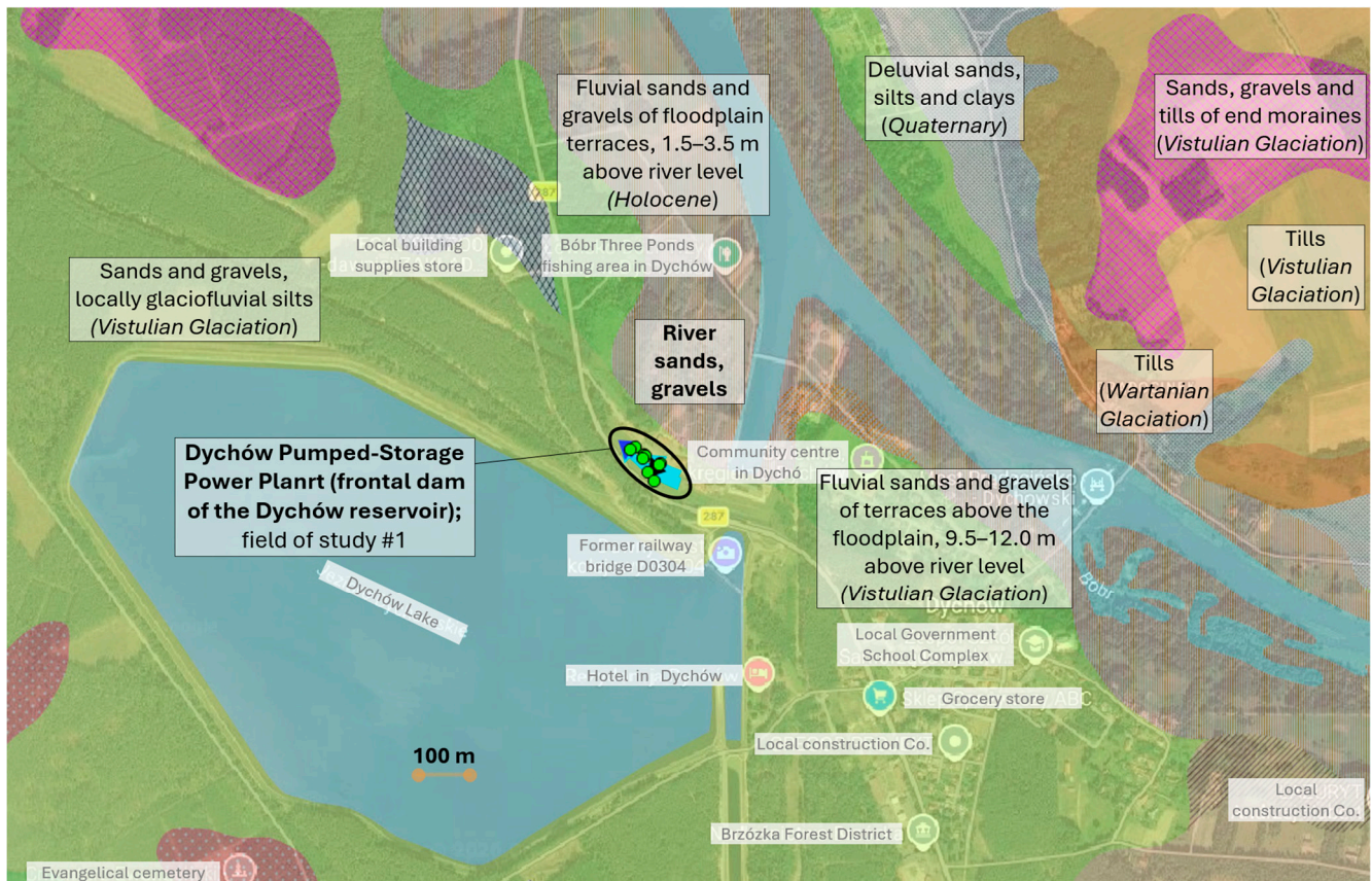
Figure 2. The location of the investigations on the lateral part of the frontal dam area of the Dychów reservoir with detailed geological map of Poland and Google satellite map in the background [24].
