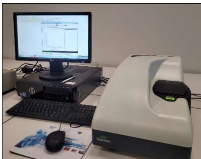
Figure 1. Zeta potential measurement setup.
