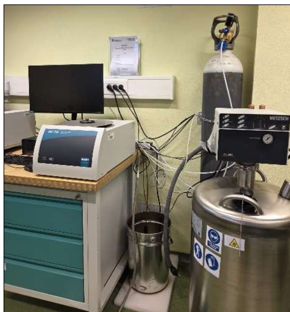
Figure 2. Measuring station for testing the heat of vaporization—differential scanning calorimeter (DSC 214 Polyma, NETZSCH).
