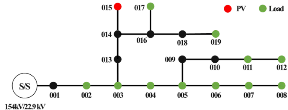
Figure 7. Simplified 19-bus equivalent test system derived from the Pyoseon DL. Red and green circles indicate PV and load buses, respectively, while black circles denote buses without PV or load connections.
