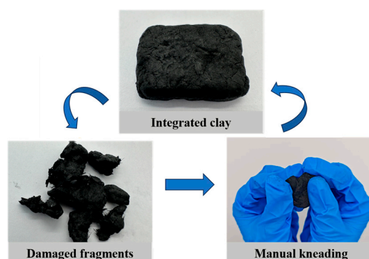
Figure 1. Mechanical reconstruction of SWCNT thermoelectric clay. The arrows indicate the sequence from integrated clay to damaged fragments, followed by manual kneading and reconstruction into an integrated form.
