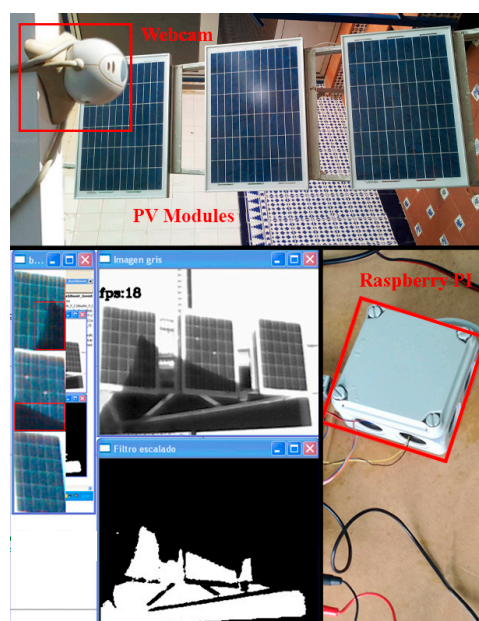
Figure 5. Vision-based MPPT implementation using a webcam and Raspberry Pi.
