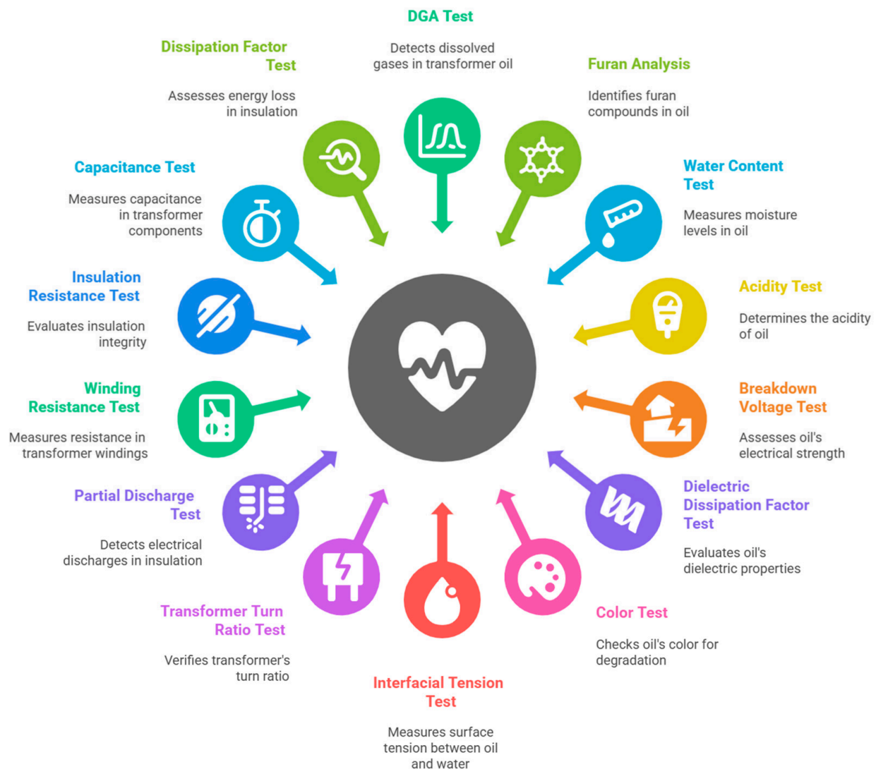
Figure 4. Diagnostic parameters of the transformer.
