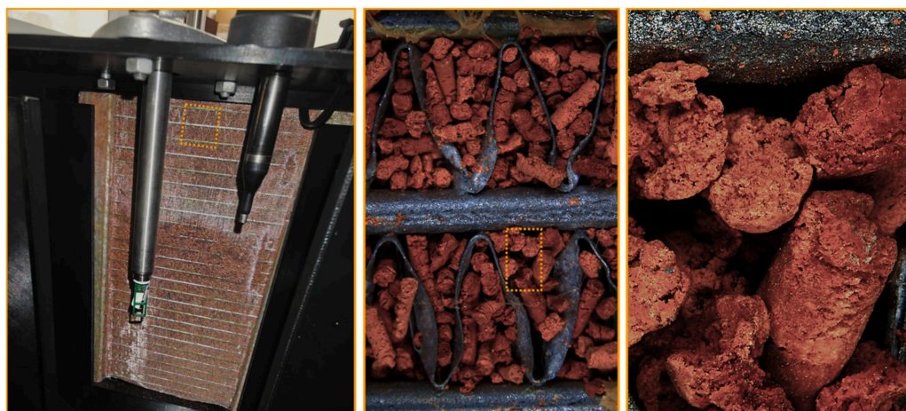
Figure 6. Picture of the tested MOF inside the heat exchanger. The orange boxes are shown at higher magnification.
