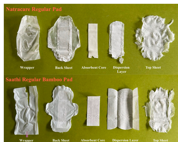
Figure 1. Reverse-engineered examples of Natracare Regular Pad and Saathi Regular Pad. Each dissected menstrual pad depicts the top sheet, dispersion layer, absorbent core, and back sheet. Pad wrapping included as well.
