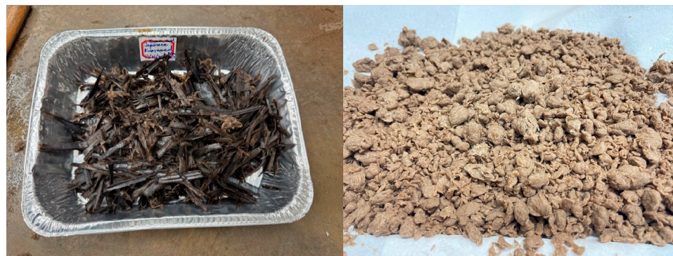
Figure 8. Japanese knotweed after Kraft cooking ( left ) and resulting brown pulp ( right ). (photo courtesy of Redmond Lab [18]).
