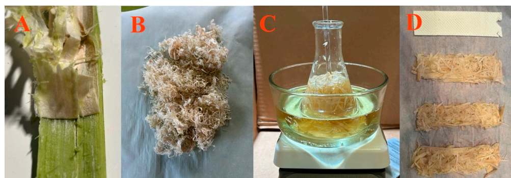
Figure 4. Chronological order of knotweed processing. Inner lumen was peeled directly from knotweed stalk (A) until enough knotweed was collected (B), then transferred to delignification bath (C). After rinsing, the fibers were pressed into the shape of an absorbent core and placed in the oven (D).
