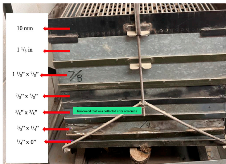
Figure 6. Williams Classifier used for chip size selection (photo courtesy of Redmond Lab [18]).
