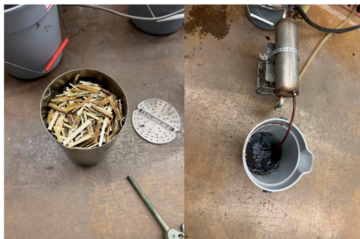
Figure 7. Japanese knotweed chips loaded into the digester (left) and black liquor collection after Kraft cooking (photo courtesy of Redmond Lab [18]).
