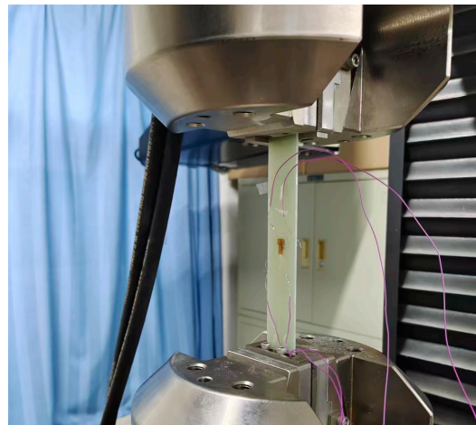
Figure 3. \pm 45^\circ shear test of glass fiber composite material.
