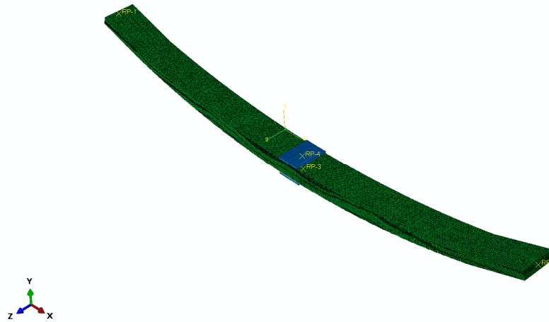
Figure 7. Finite element model of the leaf spring body.
