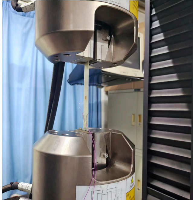
Figure 1. Tensile test fixture for 0^\circ/90^\circ layups of glass fiber composite specimens.
