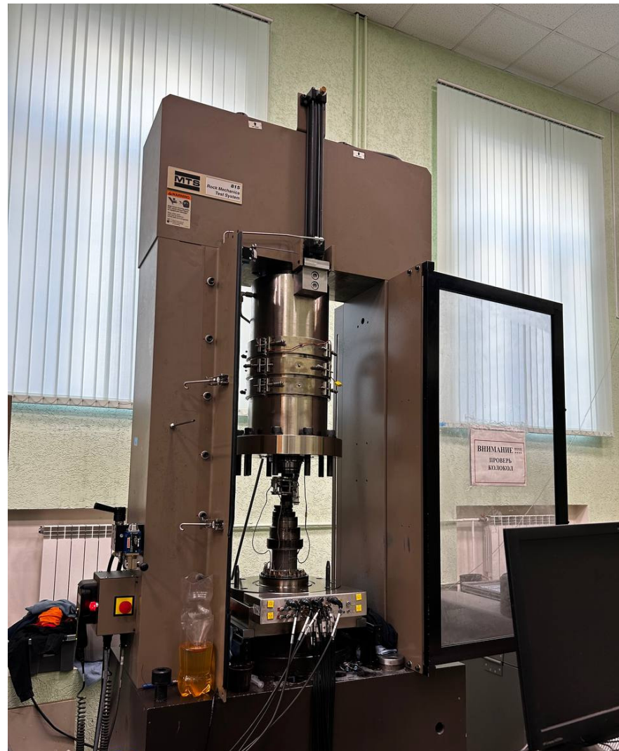
Figure 2. MTS 815 Servo-hydraulic testing machine [compiled by the authors].
