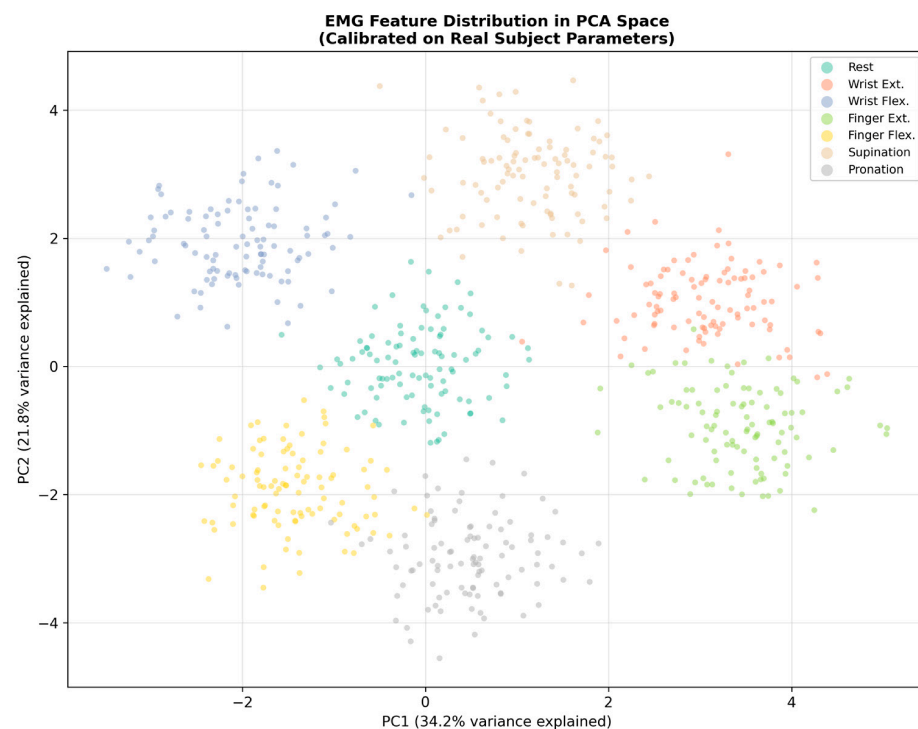
Figure 3. PCA projection of the 56-dimensional feature space showing clear cluster separation between the seven gesture classes.
