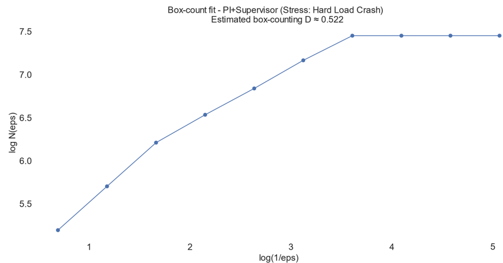
Figure 10. Box-counting fit of the PI + Supervisor error phase portrait during hard load crash, yielding an estimated fractal dimension D \approx 0.522 .
