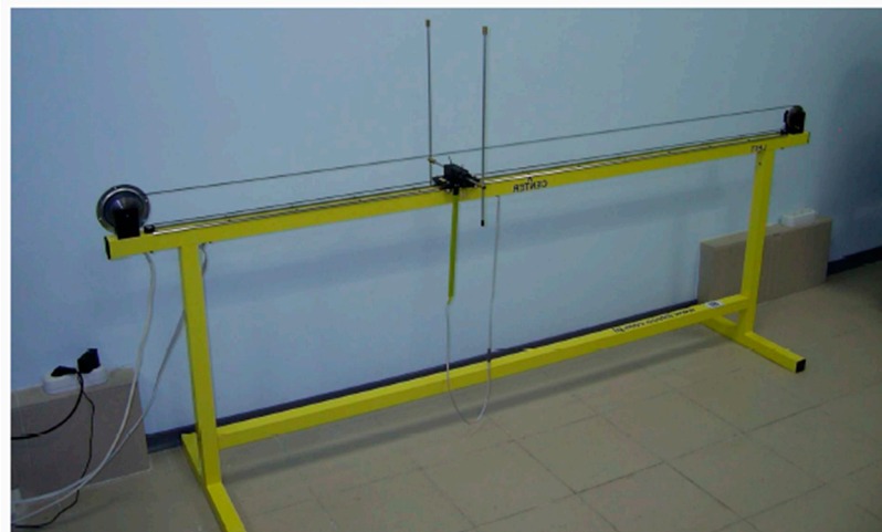
Figure 1. The inverted pendulum laboratory model.
