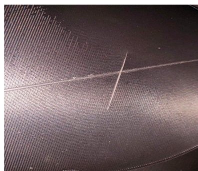
Figure 7. The crack of a notched sample.
