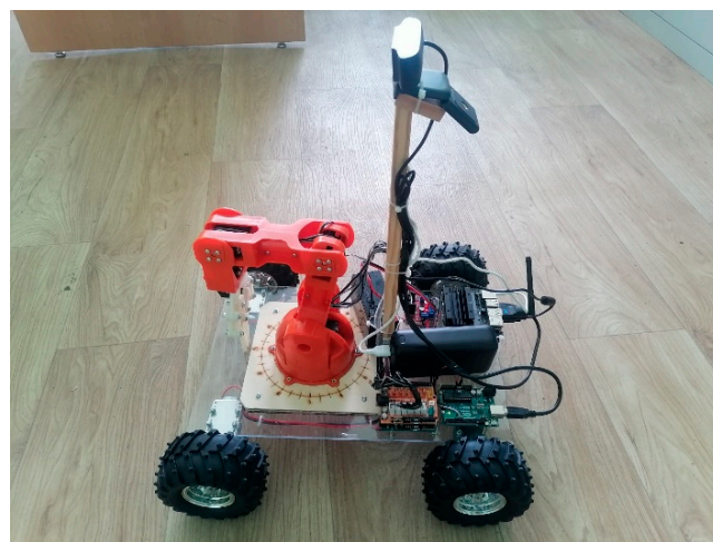
Figure 1. The developed mobile platform with a 6 DoF arm.
