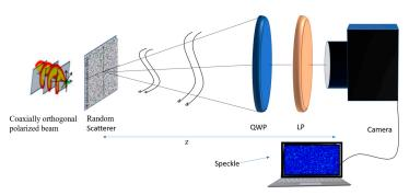
**Figure 1.** Schematic representation of proposed method. QWP—quarter wave plate; LP—linear polarizer. The CCD records intensity speckle patterns at the observation plane. These speckle patterns are used to determine two SPs.
