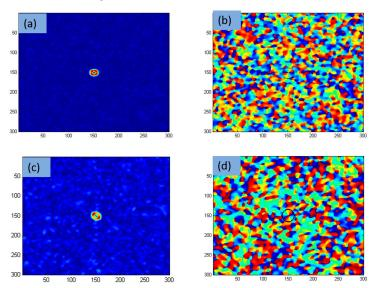
**Figure 2.** Simulation results: (a) amplitude distribution and (b) corresponding phase distribution for vortex beam with a charge of l = -1; Experimental results: (c) amplitude distribution and (d) corresponding phase distribution for the vortex beam with l = -1.
