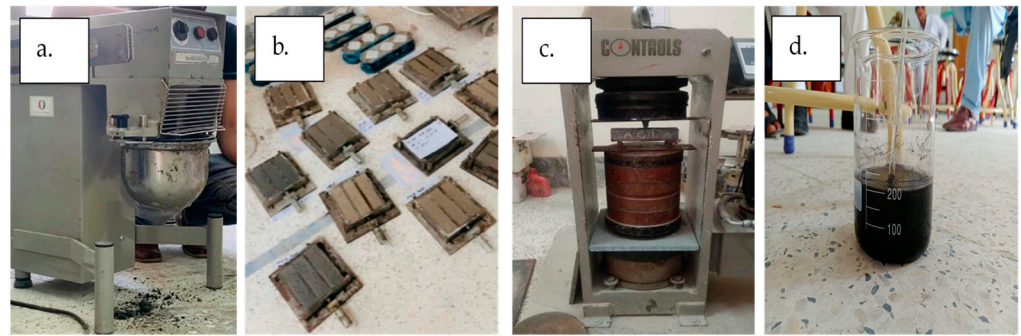
Figure 2. (a) Mixing, (b) molding, (c) flexural strength test and (d) UV-sonicated solution.
