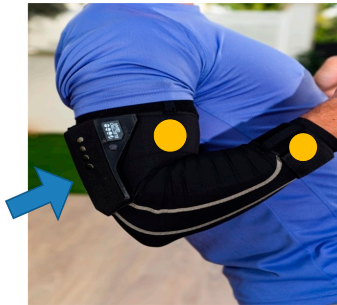
Figure 1. Blue arrow points to ElectroGear® Electron Stream® (Colchester, UK) device docked on e-textile sleeve with embedded proprietary dry microcurrent electrodes (yellow circles) and stretchable conductive pathways (grey tracks).
