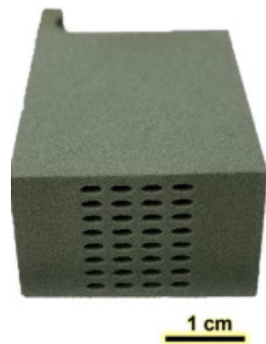
Figure 3. The prototype binder-jetting printed SiC ceramic heat exchanger's green body [16].
