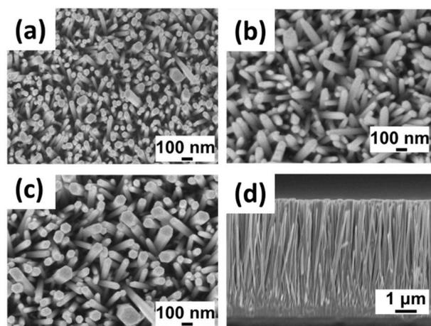
**Figure 3.** Plane SEM images of ZnO nanorods with the catalysts of (a) sodium hydroxide, (b) ammonium hydroxide, and (c) hexamethylenetetramine, and the cross-sectional SEM images of ZnO nanorods with hexamethylenetetramine (d).
