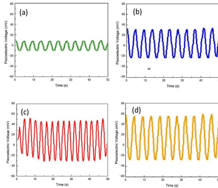
**Figure 4.** Comparison of piezoelectric sensing voltages of the ZnO nanorods tactile sensors with (a) sodium hydroxide, (b) ammonium hydroxide, (c) hexamethylenetetramine, which (d) is the polyvinylidene fluoride/ZnO nanorods with hexamethylenetetramine.
