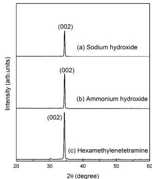
**Figure 2.** X-ray diffraction pattern of ZnO nanorods with catalysts of (a) sodium hydroxide, (b) ammonium hydroxide, and (c) hexamethylenetetramine.
