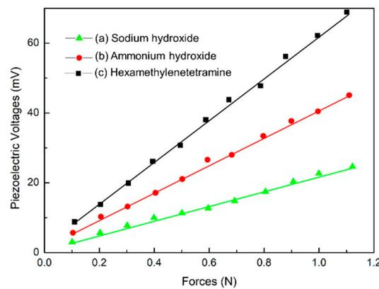
**Figure 5.** Piezoelectric sensing voltage of the polyvinylidene fluoride/ZnO nanorods tactile sensors with different catalysts under different pressures.
