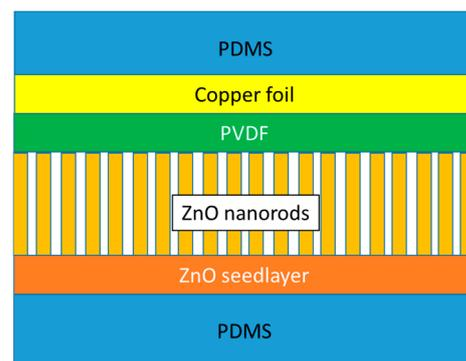
**Figure 1.** Structure of polyvinylidene fluoride/ZnO nanorod tactile sensor.
