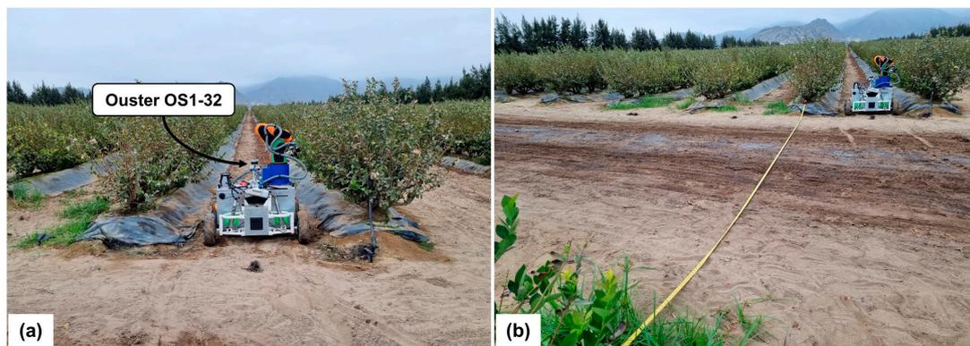
**Figure 2.** Wheeled mobile robot at the blueberry farm. (a) The robot in its initial position within an inter-row space. (b) The robot transitioning between blocks of crops and the separation between these marked with a yellow measuring tape.
